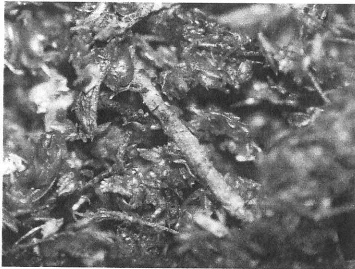
Figure 3. Close-up of largely undecomposed peat (von Post value of H1) showing the numerous lengths of moss stem and branch spindles set within the matrix of loose leaves.
